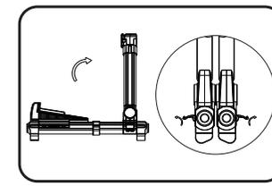
3. Move the supporting arms forward to the stop block and lock. The supporting bars adjustable back and forth to a certain space for different instruments.
