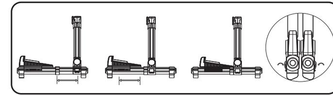
4. Open the whole stand to be A shape and place it on a horizontal surface. Place your instrument on the stand.
