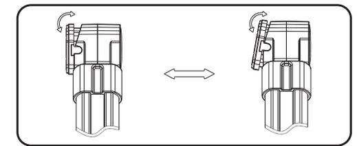
The open-close mechanism is another one patented. The mechanism ensures both arms open and close simultaneously, which improves stability of the whole structure of stand.
